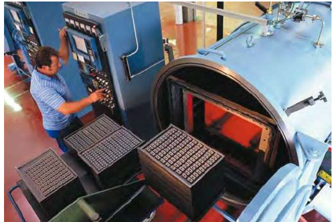
Plasma vapour deposition (PVD). Worker adjusting the controls of a PVD machine which is being used to coat components (trays at lower centre and lower left) with a thin film metal alloy to provide a wear-resistant coating.
